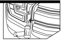
Remove the final bolt to release the headlight housing.
