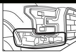
Ensure the plastic reinforcement is loose, it is not required to remove the part from the vehicle as a whole unless needed.
