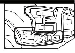
Replace the bolts to secure the plastic reinforcement.
