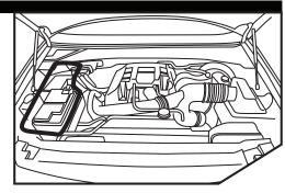
Install the Aura Control Box by connecting the positive wire for a constant on functionality (always on when battery is on) or an accessory wire (only on when the vehicle is on) which can be found in the Fuse Box. Connect the negative wire to a ground wire.
