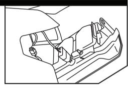
Install new headlight housing by connecting the electrical harness.
