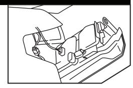
Unplug the electrical harness from the back of the headlight housing.
