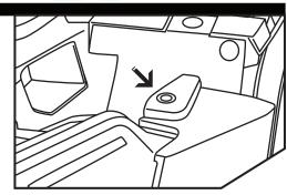
Secure the trim by inserting the plastic clip and locking into place.
