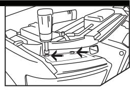
Remove the two bolts on top of the headlight housing using the screwdriver.
