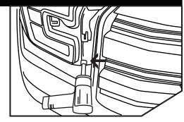
Replace the bolt to secure the headlight.
