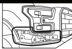
Remove the bolts holding the plastic reinforcement.
