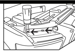
Replace the two bolts on top to secure the headlight housing.
