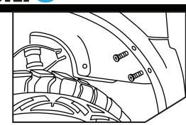
Remove the 2 bolts in the wheel well.
