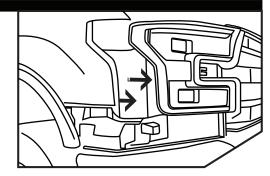
Pull the front of the projector headlight towards you to remove the headlight housing from the vehicle.
