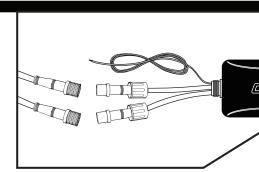
Connect the round connector from the headlight housings to the control box.
