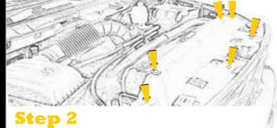
Remove the plastic retainers securing the filler panel – there should be 6 in total.
