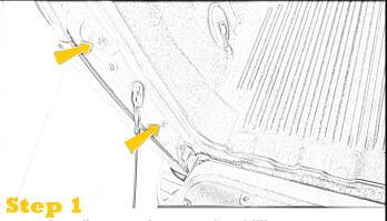
Open the tailgate, and remove the Phillips screws holding the stock tail light (2 total).
